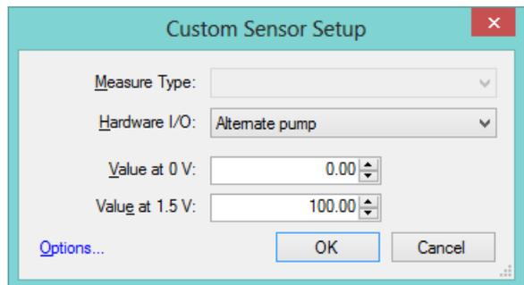
The selected sensor is displayed in the **I/O** (input/output) column, which is **15A**, **75A** or **Alternate** for all other types of sensors. Place the pump input switches (next page) at the proper positions on the device (15A, 75A, ALT) by means of a small screwdriver or a paperclip.
