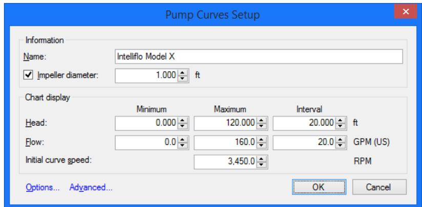
To create pump curves, enter the minimum and maximum values for the X-axis (flow) and Y (head) from the pump curve graph (like on the previous page) and the value of the intervals in the appropriate fields. Set a speed at which the first curve will be created in the **Initial curve speed** field. Start by the highest RPM curve.
