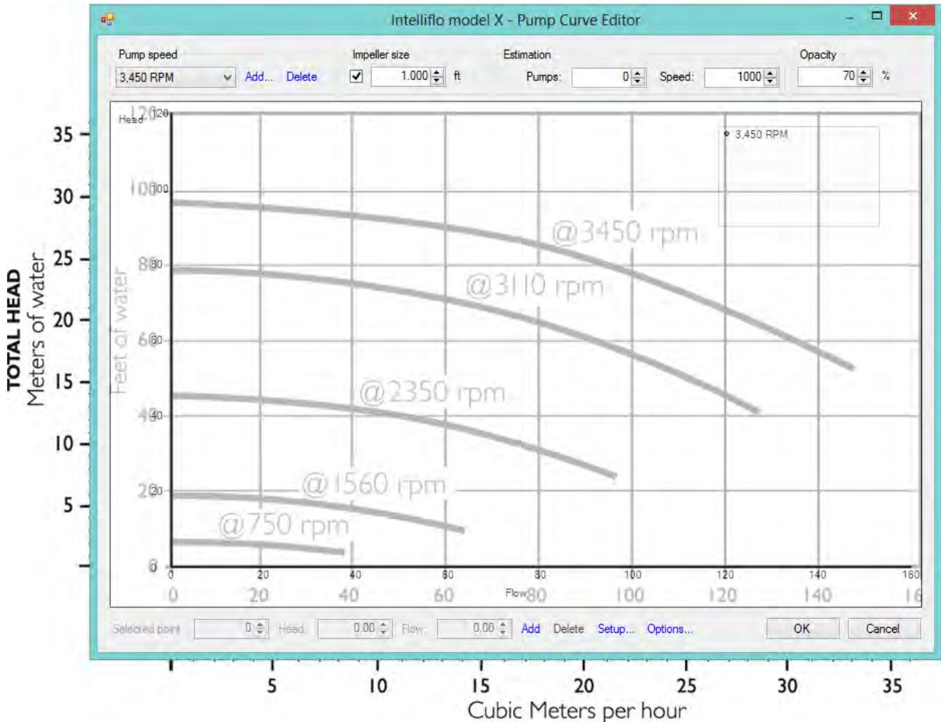
When overlapping the windows, be sure to use identical scales and adjust the window size for a perfect overlay of the graph of the pump curve document. Place the origin of the axes over each other to start and stretch the top and right sides of the **Pump Curve Editor**.
