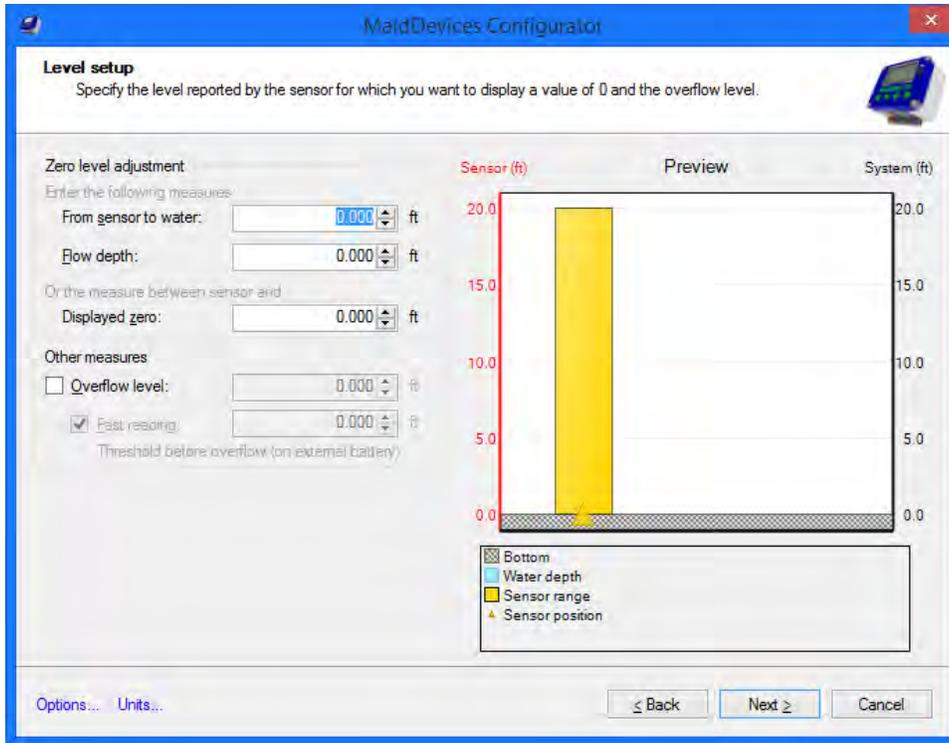
If a level sensor is configured at the **Inputs and outputs page**, the Level setup dialog will be displayed and a graph will show the range of the sensor with other options like the possibility to record sewage sewer overflow events including volume lost during the event.
