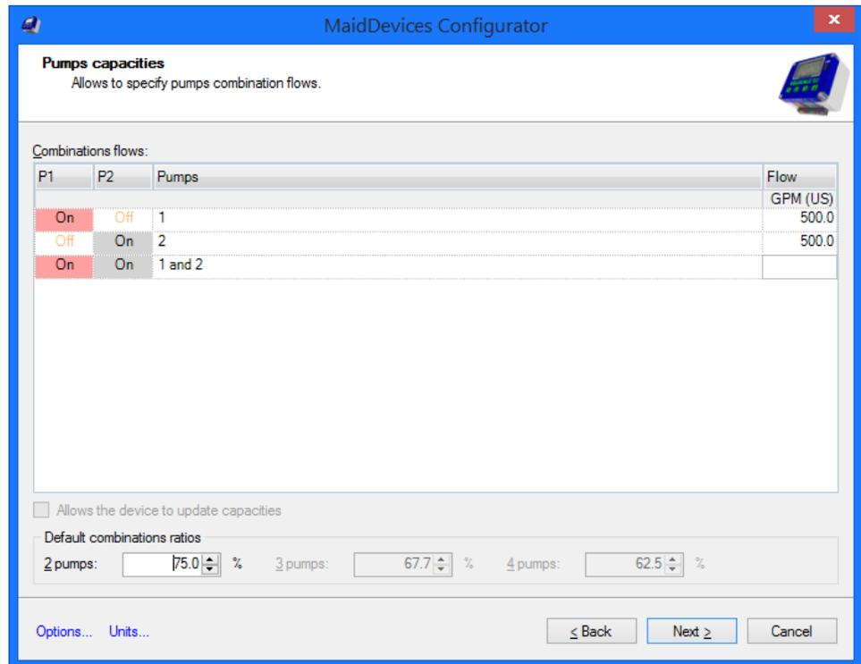
**Pumps curves** can be used as the **Flow algorithm** for fixed and variable speed pumps. Other than being connected to an external flow meter, this is the only mean to calculate the flow out of variable speed pumps.
