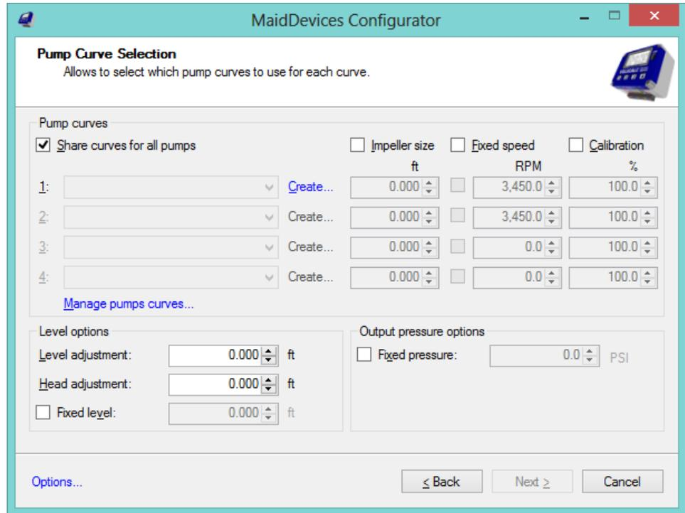
The pump curves are usually provided free from the manufacturers. They represent flow rate relative to the head condition. Variable speed pumps have several curves in the graph for multiple RPM. Note: Before creating curves in the Configurator, it is important to have these curves in the computer and in a graphic format. The pump curves images should be displayed in a large format. Here is an example of pump curve : Model INTELLIFLO
