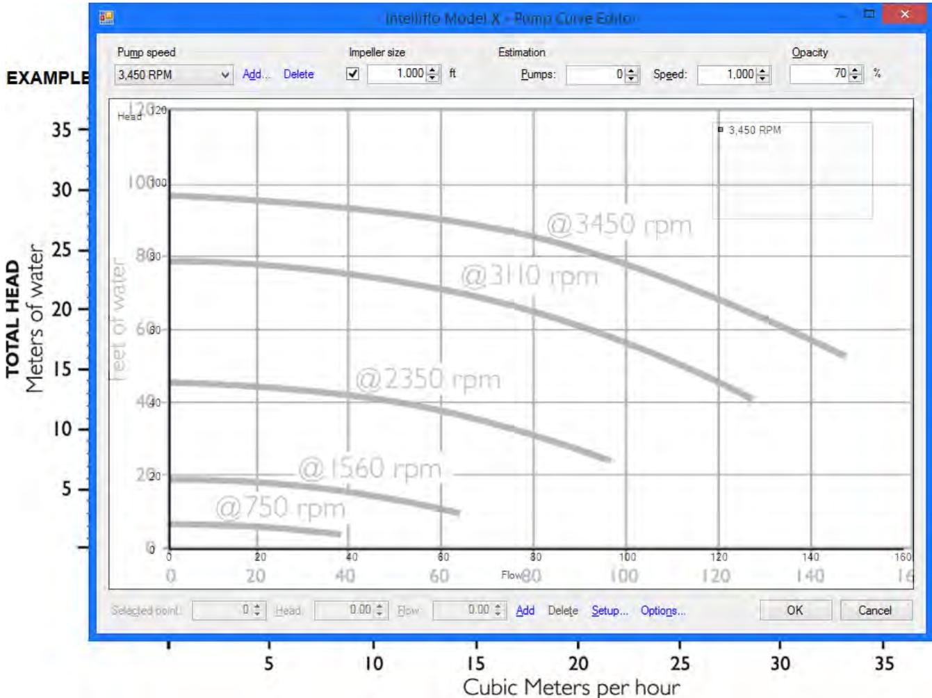
When overlapping the windows, be sure to use identical scales and adjust the window size for a perfect overlay of the graph of the pump curve document. Place the origin of the axes over each other to start and stretch the top right sides of the **Pump Curve Editor**.
