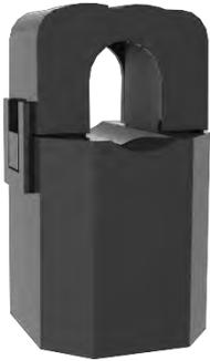
The Split-core current transformer MLCT75 is designed to provide a low-cost method for monitoring electrical current. Its unique hinge pressure locking mechanism enables its installation without interrupting the current supply to the pumps or equipment.
