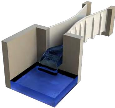
The Parshall weir is available in several sizes. Dimensions directly supported by the device are those in the following table. In the case where the size of the weir is not available in the table, just use the standard formula and set the parameters for the equivalent.
