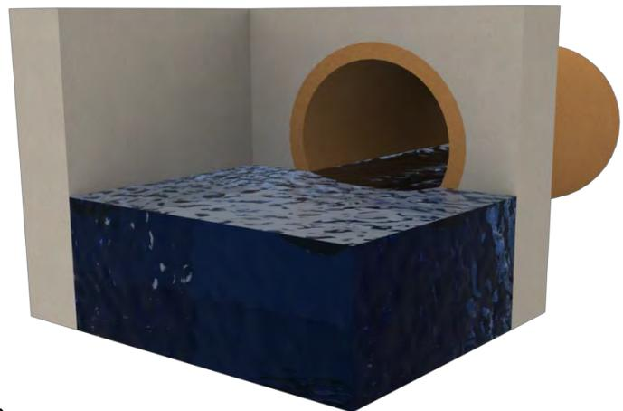
The Manning equation is used to estimate the flow in open channel situations where it is not practical to construct a weir or channel to measure the flow with greater accuracy.
