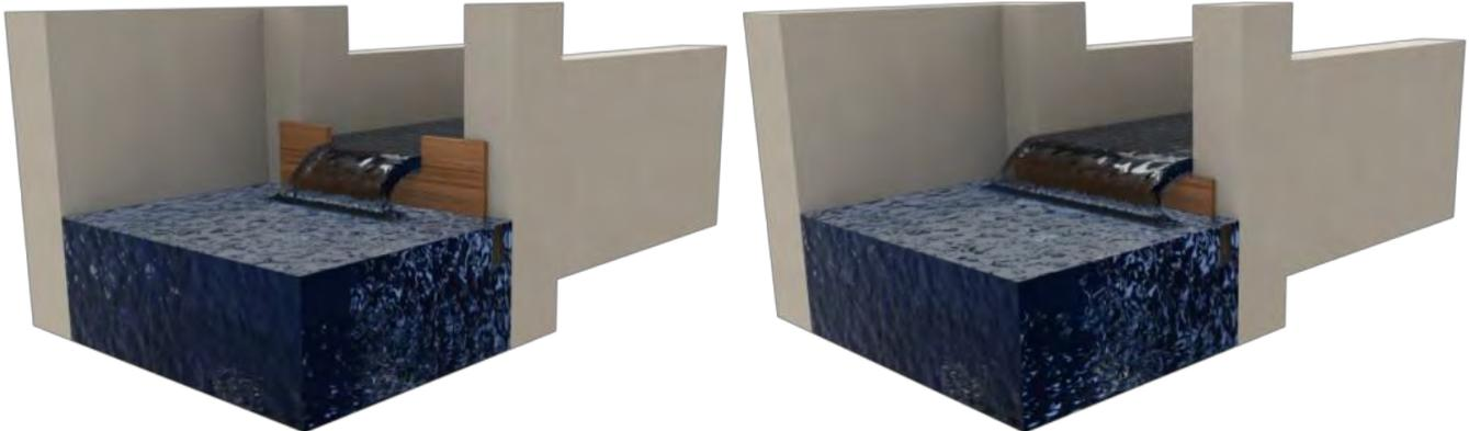
The accuracy of rectangular weirs, with or without contractions, is usually between 1 to 4% of the flow coefficient when all conditions are met.
