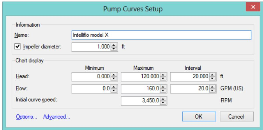
When the diameter of the impeller is known, it can be entered as part of the curve. If a different impeller diameter is used and entered in the Pump Curve Selection dialog (previous page), then the calculate flow will be automatically adjusted according to updated data on the impeller's diameter.  Impeller size ft 0.000
