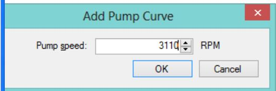
curve, it is recommended to do a curve scan using the dotted curve created in the **Estimation** section (top right). In the **Pumps** field, enter 1 and then change the **Speed** using the arrows. The dashed
