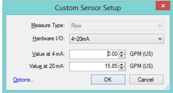
The 4-20 mA loop is powered by internal 12VDC. No external power is required.
