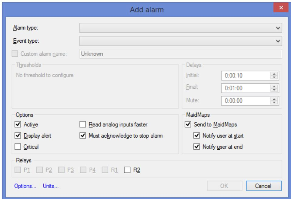
**Must acknowledge to stop alarm** is used to display the alarm on the device and require a user to acknowledge it or it will always stay on top.
