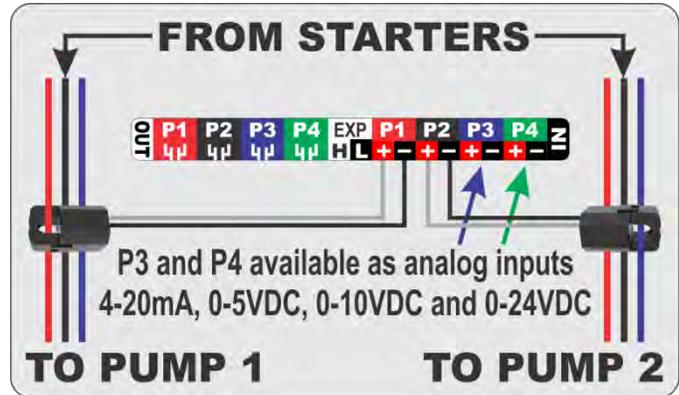
If mini current sensors (MLCT75) are used for pumps of less than 10 HP, then the DIP switches should be moved left with a very small screw driver or a paper clip to adjust the setting of the current clamp to 15 Amps.
